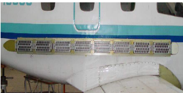
Figure 5. A system for shooting pyrotechnic PV-26 flares
