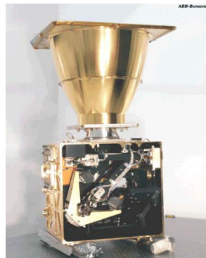
Solar-occultation Fourier Transform Spectrometer (FTS) based on the Atmospheric Chemistry Experiment FTS on SCISAT
