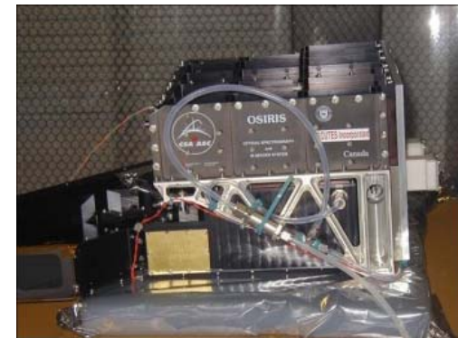
Limb-scanning atmospheric scatter instrument (CATS) based on the Optical Spectrograph and Infra-Red Imaging System (OSIRIS) on Odin
