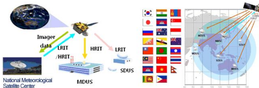
Fig. 2. Concept of MI H/LRIT direct broadcasting
