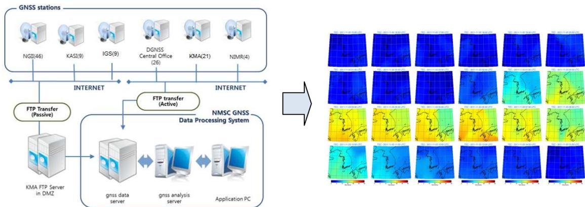
Fig. 1 KMA GNSS data processing system (Left) and TEC map over Korea (Right)
