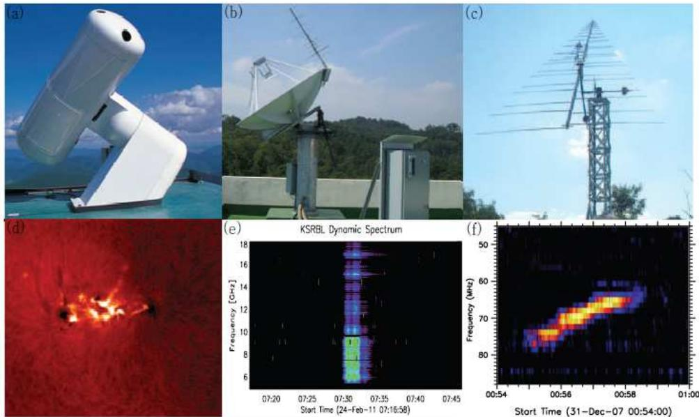
**Figure 1.** Representative solar observational systems and data in Korea. (a) Solar Flare Telescope (SOFT), (b) Korean Solar Radio Burst Locator (KSRBL), (c) e-CALLISTO, (d)  $H\alpha$  flare observed by SOFT on 15 Feb. 2011, (e) Solar radio burst observed on 24 Feb. 2011 by KSRBL, and (f) type II radio burst observed on 31 Dec. 2007 by e-CALLISTO.
