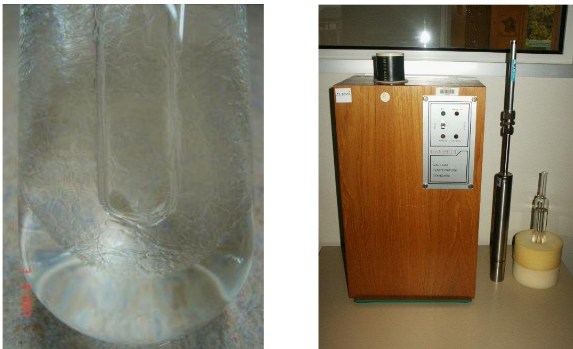
Figure 1: Triple point of water cell ready to use and fixed point cells (Météo-France) gallium, mercury and water
