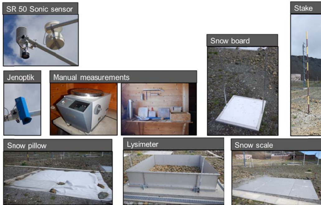
Figure 4: The snow on the ground measurements at Weissfluhjoch SPICE site.
