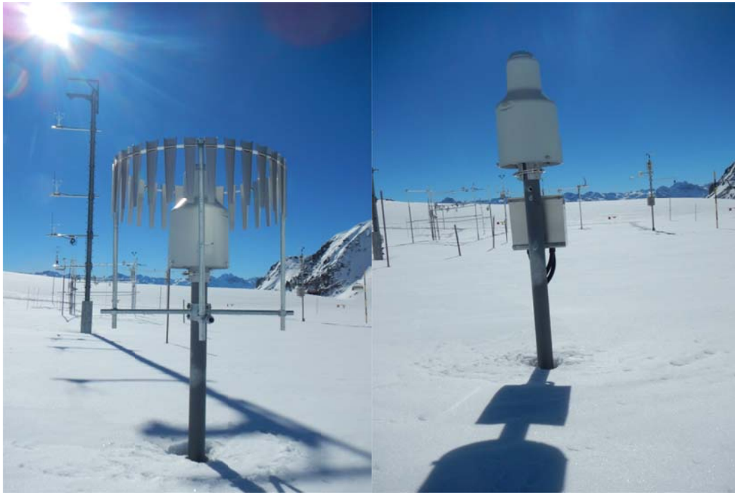
Figure 3: The R3 SPICE reference with one Pluvio 2 unshielded (right) and one with a Single Alter shield (left)
