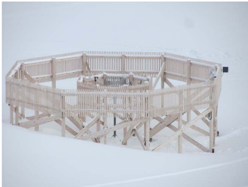
Figure 2: The R2 SPICE reference with a Pluvio 2 in a Single Alter shield surrounded by a DFIR (Double Fence International Reference)
