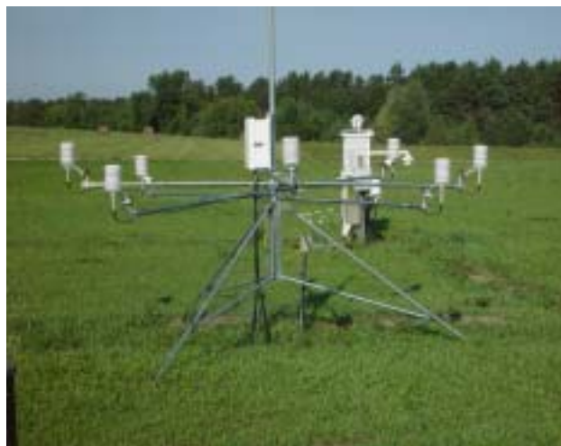
Figure 2 - Test sensors in Gill 12-plate screens
