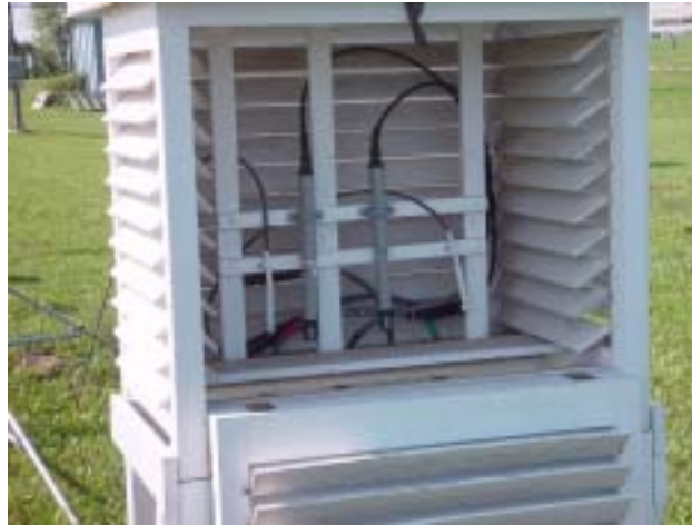
Figure 1 - Test sensors in non-aspirated Stevenson screen.
