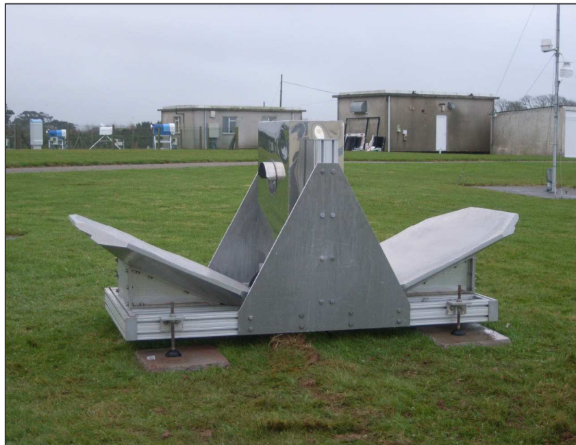
Figure 1 – Cloud radar front-end deployed at Camborne Met office, UK. The Jenoptik Lidar used for comparison can also be seen in the background (grey rectangular unit near the left edge of the figure).
