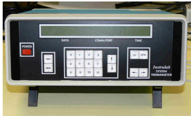
Figure 4. Instrulab 4312 PT100 temperature Indicator
