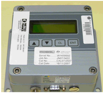
Figure 2. Vaisala PTB220A barometer
