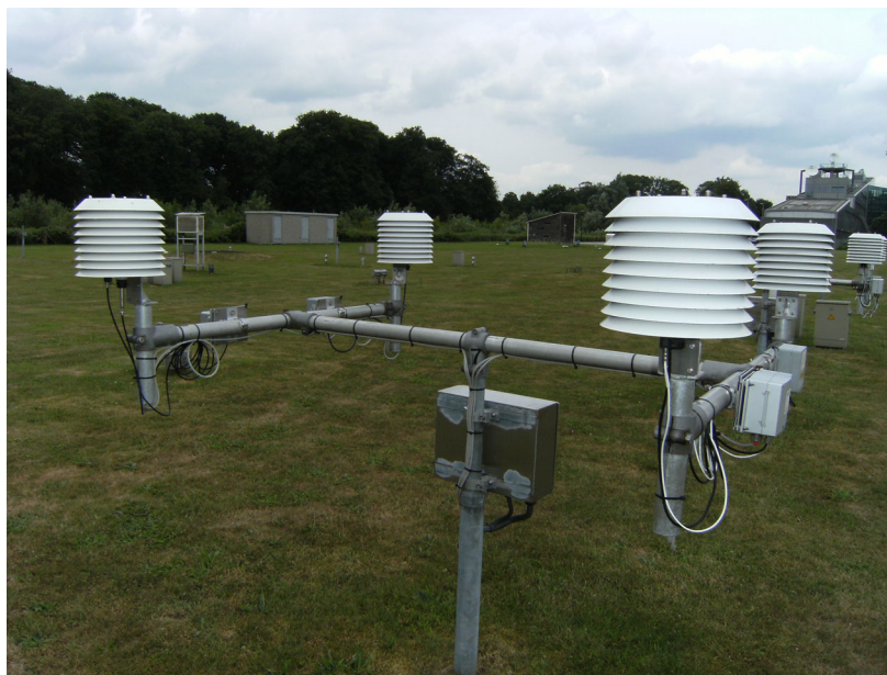
Figure 4. The field test in De Bilt. Shown are the radiation screens containing the humidity sensors.
