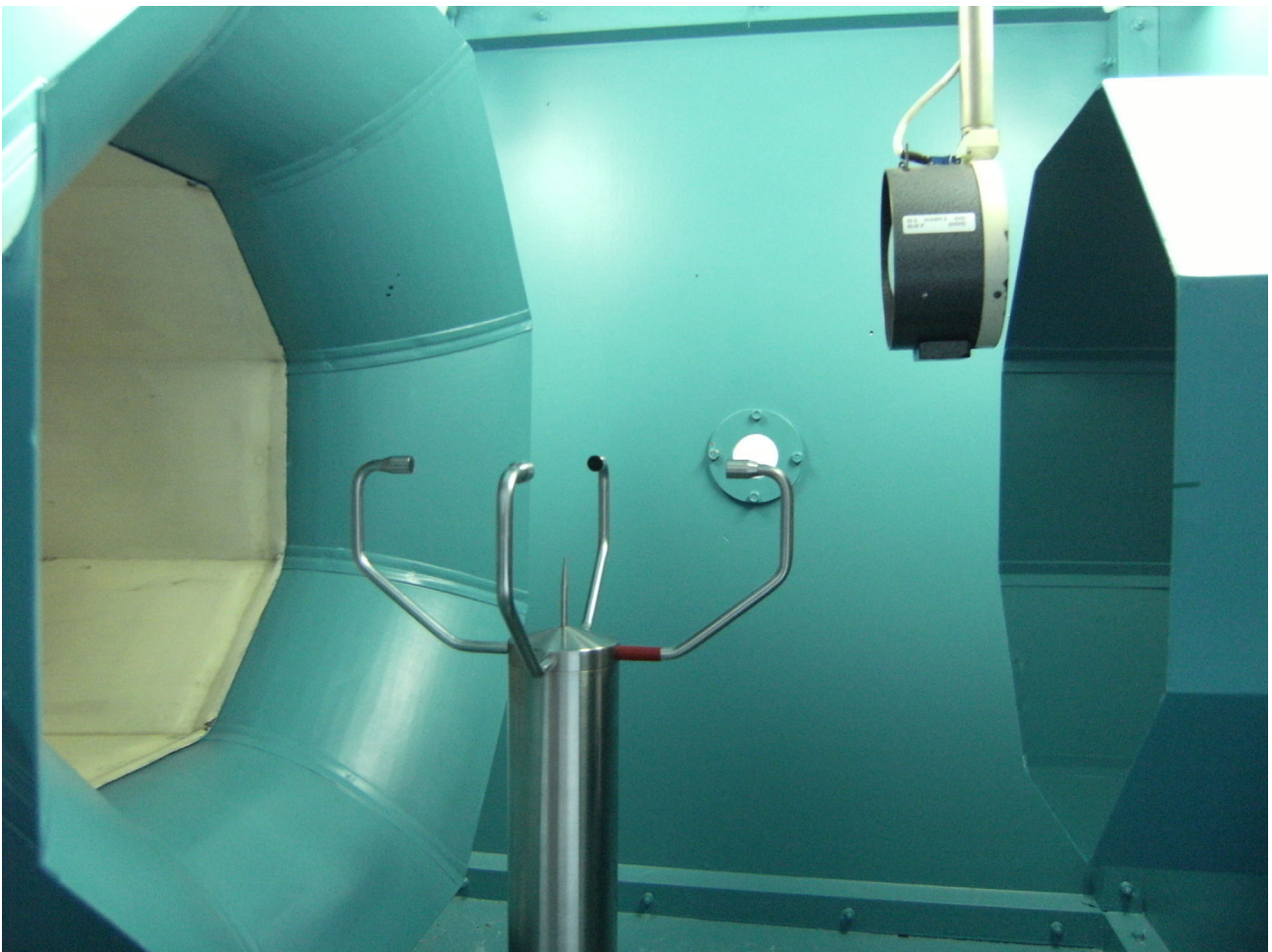
Figure 1: A Thies 2D sonic wind sensor in the measurement section of the KNMI wind tunnel.
