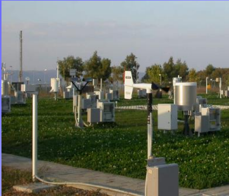
Young 05106 wind sensors + Vaisala DRD11A Rain detectors (USA)
