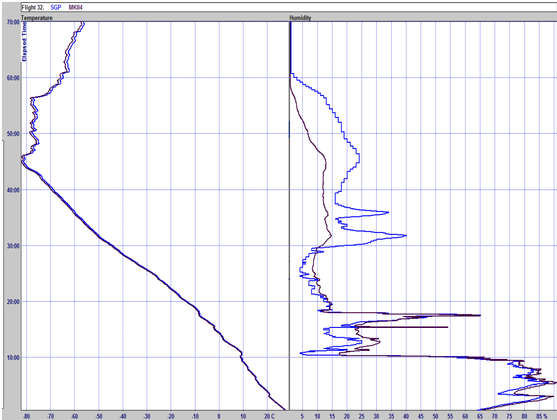
Fig. 14 Simultaneous measurements of temperature and relative humidity, Sippican MkII and Vaisala RS92 (SGP)
