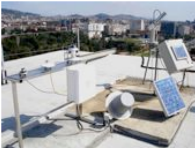
Sun photometer managed by the UPC integrated in the AERONET network
