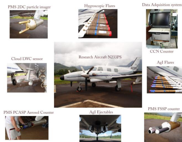
Figure 2. The Piper Cheyenne equipped for seeding and cloud physics measurements.
