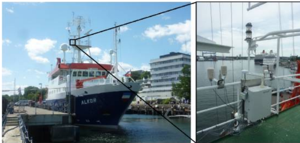
Figure 13: Installation on Alkor (DWD)
