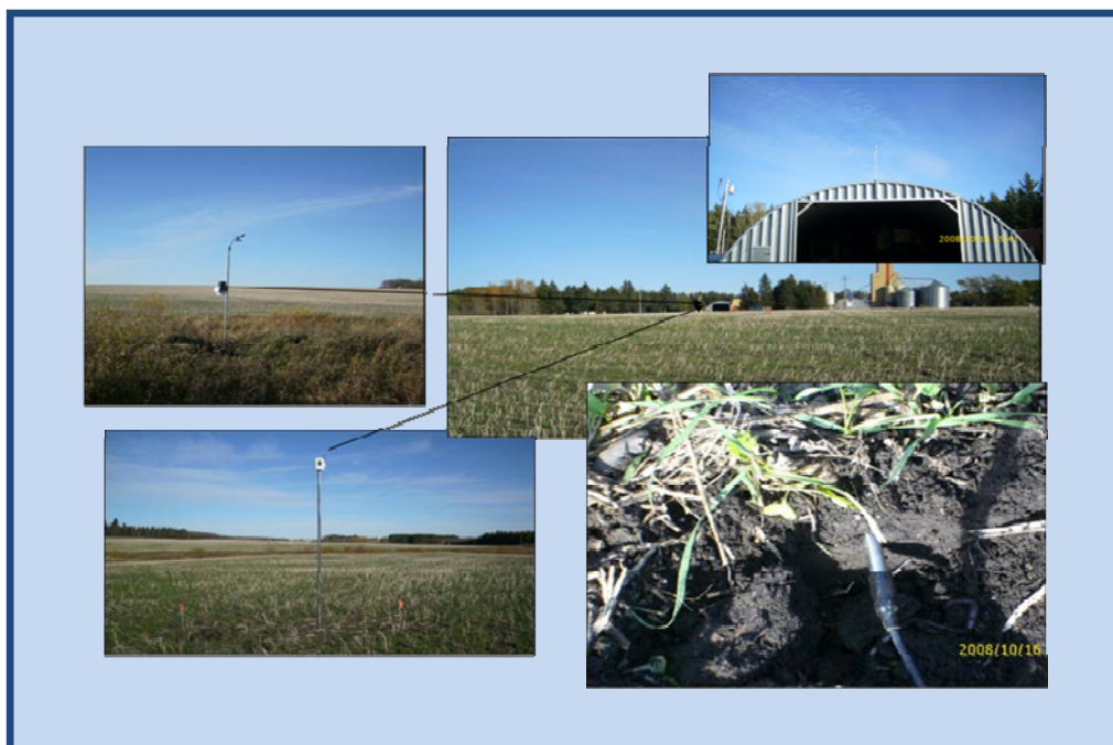
Figure 3: A typical on-farm installation. All sensors, including the weather station, update every 2.5 seconds utilizing the Internet; weather data is stored in servers in Washington, D.C. Photo source: Canadian Wheat Board.
