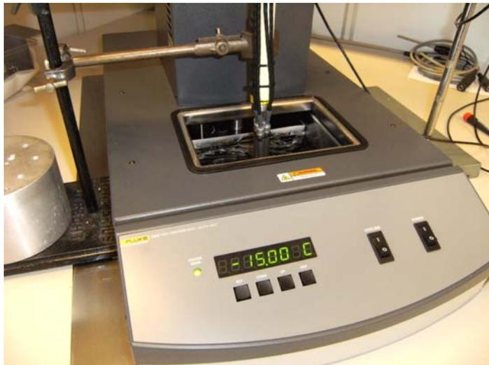
Figure 1. The calibration bath containing the sensors and the reference thermometer.
