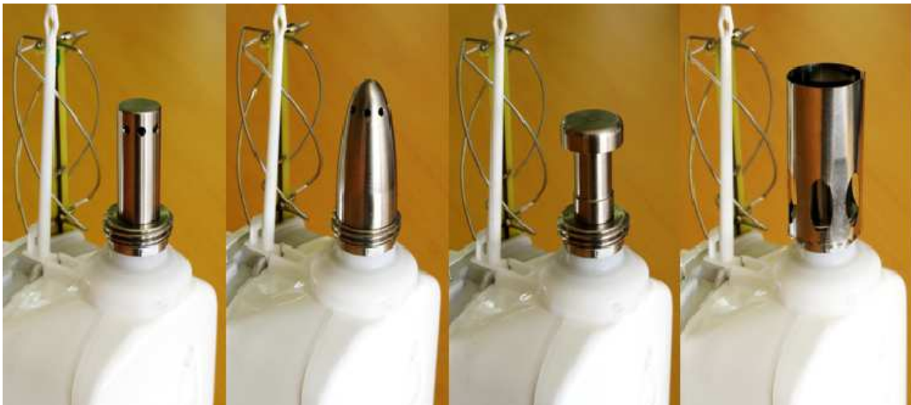
Figure 2. The three different types of wind shields and a radiation shield (on the right) used during the LAPBIAT2 campaign.
