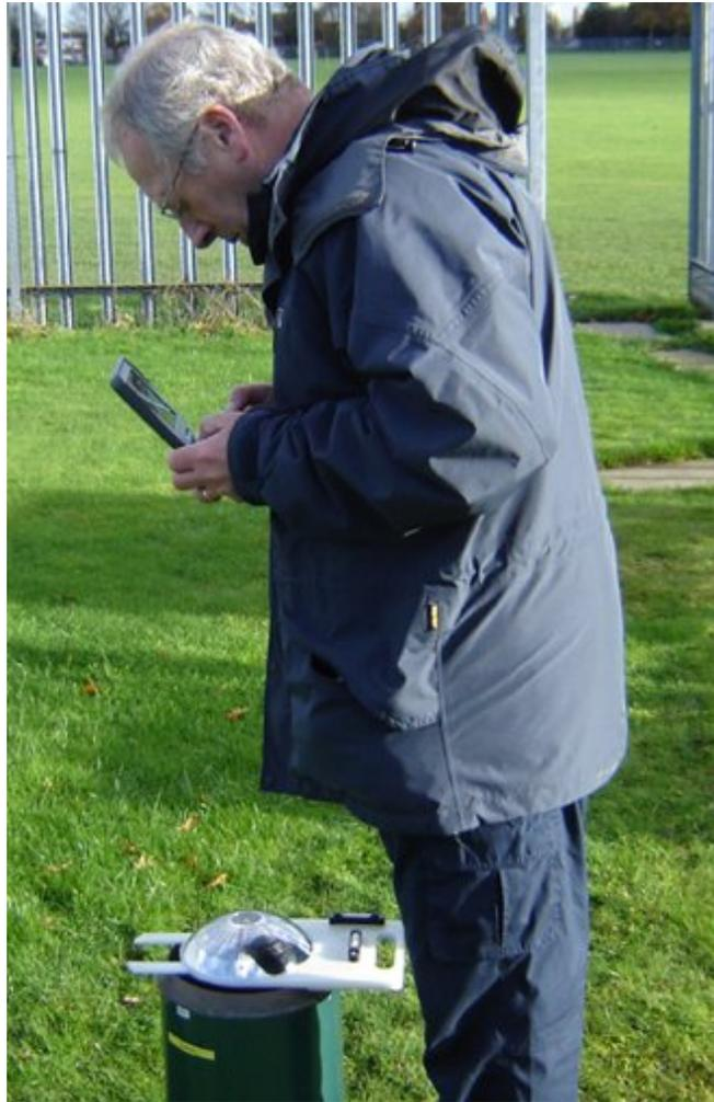
Fig 5. RNM assessing raingauge exposure and recording results.
