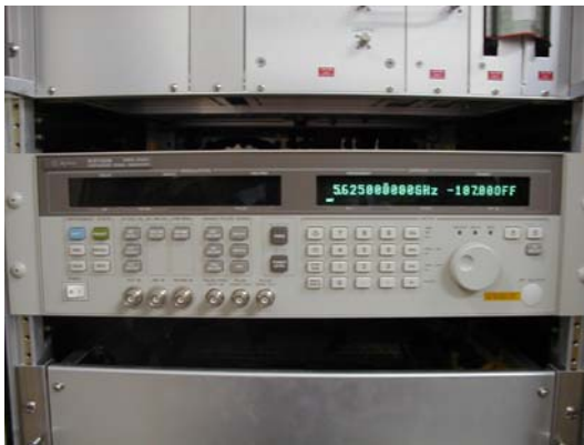
Pict. 4- Automatic Signal Generator mounted to the radar system
