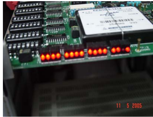
Pict. 6- Electrically adjustment by using dip switch
