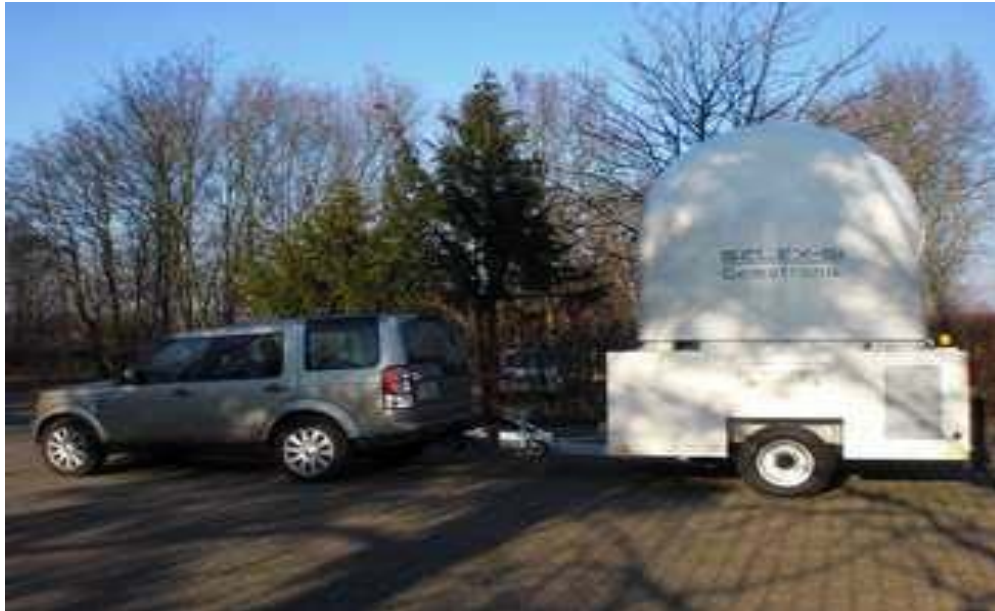
Pict.9 Mobile X-Band Radar with Magnetron tube
