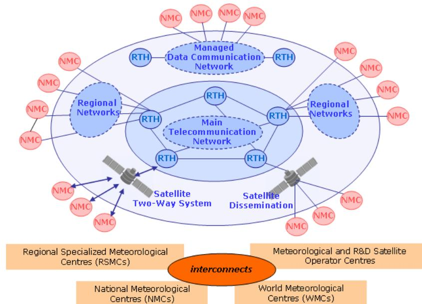
Figure 1. High-level schematic of the Global Telecommunication System (GTS) (source: [http://www.wmo.int/pages/prog/www/TEM/GTS/index\\_en.html](http://www.wmo.int/pages/prog/www/TEM/GTS/index_en.html))
