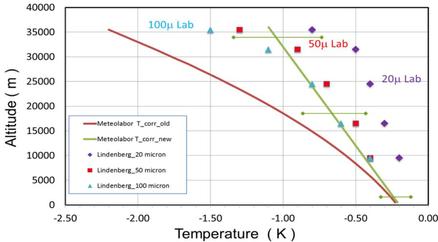
Figure 2: Old (red) and new (green) radiation error curve. The green curve is experimentally determined in flight with 50 micron thermocouples under shaded and unshaded conditions. The purple, red and blue marks are measured in the vacuum chamber using 20, 50 and 100 micron thermocouple sensors.
