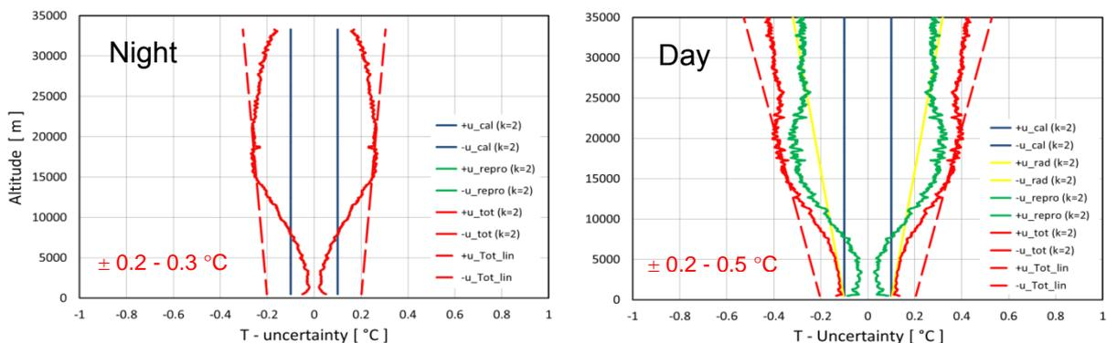
Figure 3: Night and day uncertainty estimates for SRS-C34 radiosonde temperature measurements
