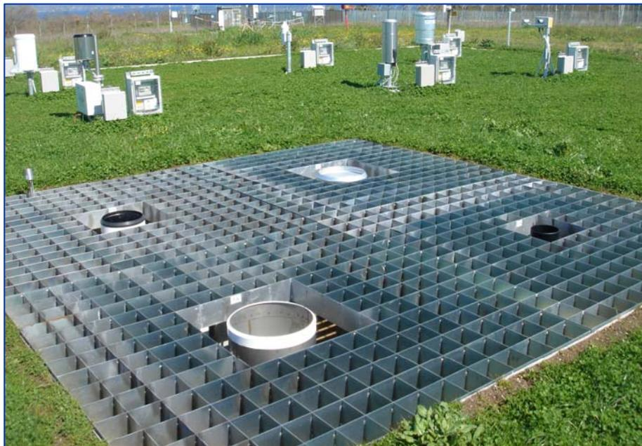
**Fig.2 – 4-fold RRGP – The 4 working reference RI gauges.**
