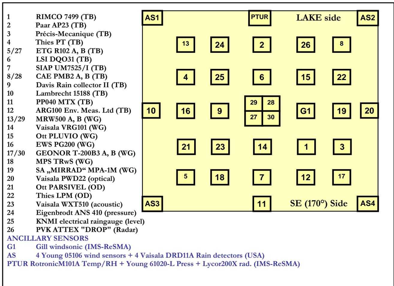
Fig.3 – WMO Field Intercomparison: Instruments Positioning
