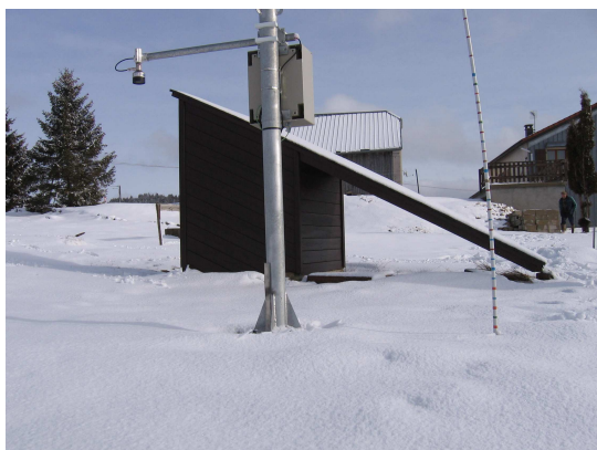
Figure 2 : Snow depth sensor Campbell SR50A and snow stick at the site of La Pesse. 17 January 2008.
