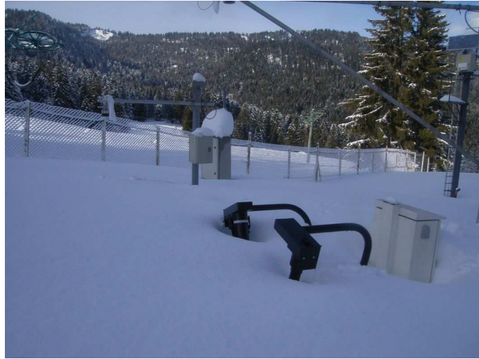
Figure 9 : Campbell SR50A and SOLIA 300 (buried under the snow) at Col de Porte, 21 January 2008.
