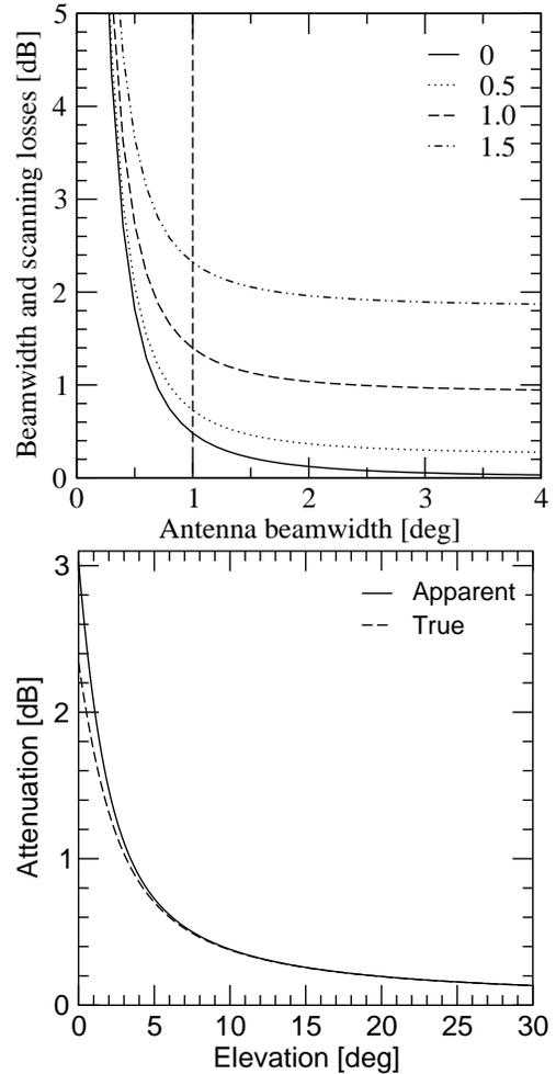
Fig. 3. The top frame shows the calculated correction for the beamwidth and the scanning losses as a function of the 3 dB width of the radar antenna. Curves for different ratios (0...1.5) of the azimuthal width of the processed rays and the 3 dB antenna beamwidth are shown. The bottom frame shows the calculated gaseous attenuation of the sun at radio frequency as a function of the apparent (solid) and true (dashed) elevation.
