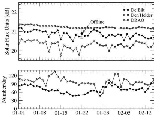
Fig. 5. Daily analysis of the sun signatures observed by the weather radars in De Bilt (filled circles) and Den Helder (open circles) from 1 January to 15 February 2008. For reference the observations from DRAO are plotted as well. The upper panel displays the solar flux and the lower panel shows the number of analyzed sun signatures per day. The result from the offline sun tracking in De Bilt on 22 January 2008 is also plotted.
