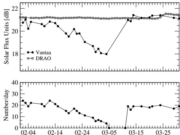
Fig. 6. Daily analysis of the sun signatures observed by the weather radar in Vantaa and the DRAO reference from 1 February to 31 March 2008. The upper panel shows the observed solar flux and the lower panel the number of analyzed sun signatures per day.
