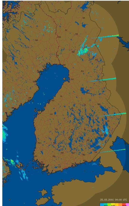
Fig. 1. Reflectivity composite from Finnish radar network with four sun signatures recorded during sunrise.
