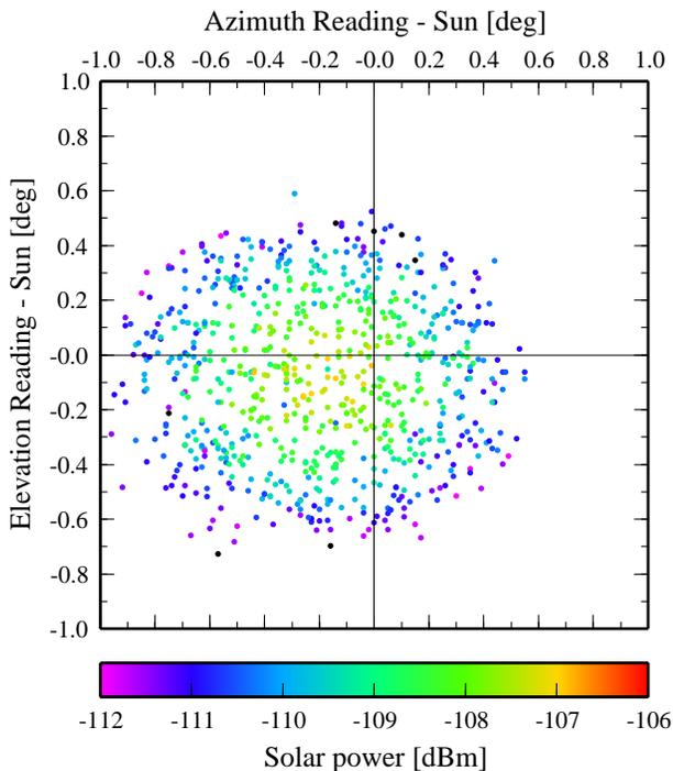
Fig. 4. A scatterplot of the solar signals collected by the weather radar in De Bilt during March 2004. The vertical axis gives the difference between the observed antenna elevation (reading) and the calculated elevation of the sun, and the horizontal axis the same for the azimuth.
