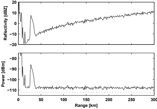
Fig. 2. Radar A-scope plot with uncorrected (top) and corrected (bottom) reflectivity signals from the sun.
